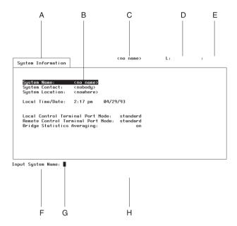
Figure 2-1 Bridge Screen Components
